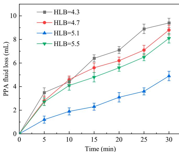
**Figure 1.** PPA fluid loss vs. time in cases of different HLB values.
