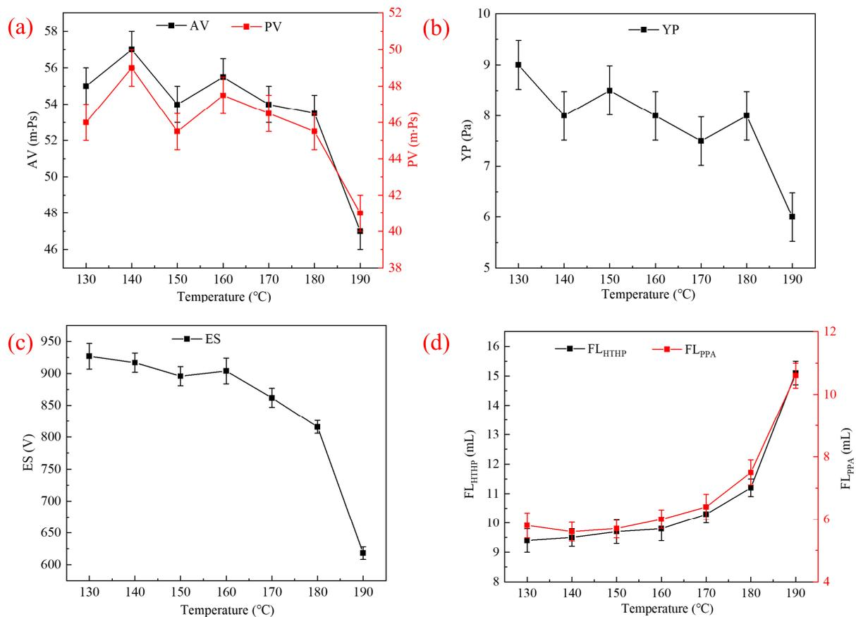
**Figure 10.** Values of (a) AV and PV, (b) YP, (c) ES and (d)  $F_{HTHP}$  and  $F_{PPA}$  after aging (AA) at different temperatures.
