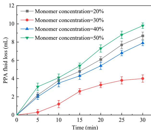
**Figure 4.** PPA fluid loss vs. time in cases of different total monomer concentrations.
