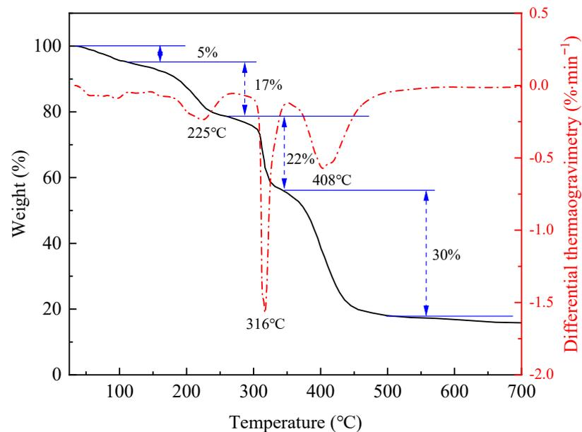
**Figure 7.** Thermogravimetric analysis of polymeric microspheres.
