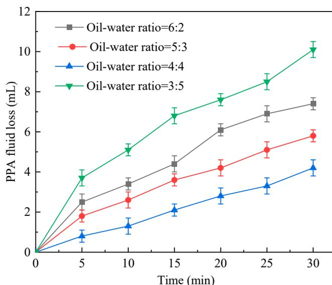
**Figure 2.** PPA fluid loss vs. time in cases of different oil–water ratios.
