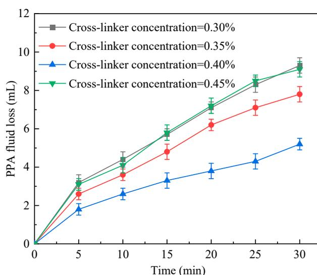
**Figure 5.** PPA fluid loss vs. time in cases of different cross-linker concentrations.
