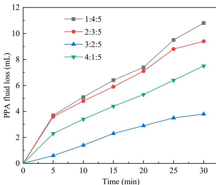
**Figure 3.** PPA fluid loss vs. time in cases of different monomer ratio (AMPS:AM:NVP).
