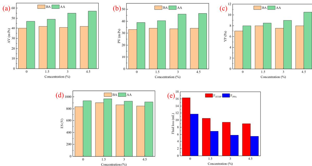
**Figure 9.** Values of the (a) AV, (b) PV, (c) YP, (d) ES and (e)  $F_{\text{HTHP}}$  and  $F_{\text{PPA}}$  of OBFs with different concentrations of AMND before and after aging (BA and AA) at  $130 \text{ }^\circ\text{C}$ .
