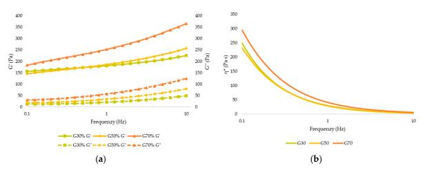
**Figure 1.** (a) Elastic modulus (G') and viscous modulus (G''). (b) Complex viscosity ( $\eta^*$ ) of the apricot gel before 3D printing (G30: Gel 30% pulp; G50: Gel 50% pulp; G70: Gel 70% pulp).
