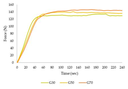
**Figure 2.** Example of force vs. time curves during forward extrusion measurement for apricot gel before 3D printing. (G30: Gel 30% pulp; G50: Gel 50% pulp; G70: Gel 70% pulp).
