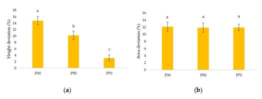
**Figure 3.** (a) Deviations of the height parameter of the samples. (b) Deviations of the area parameter of the sample (P30: Printed sample 30% pulp; P50: Printed sample 50% pulp; 70: Printed sample 70% pulp). Letters (a–c) indicate homogeneous groups according to ANOVA (p < 0.05).
