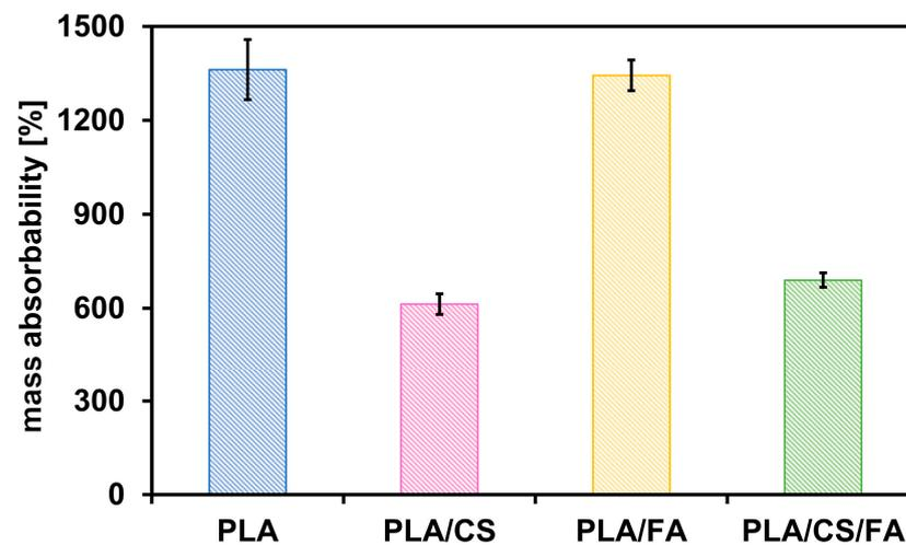
**Figure 7.** Mass absorbability values of the scaffolds. Error bars represent the standard deviation values.
