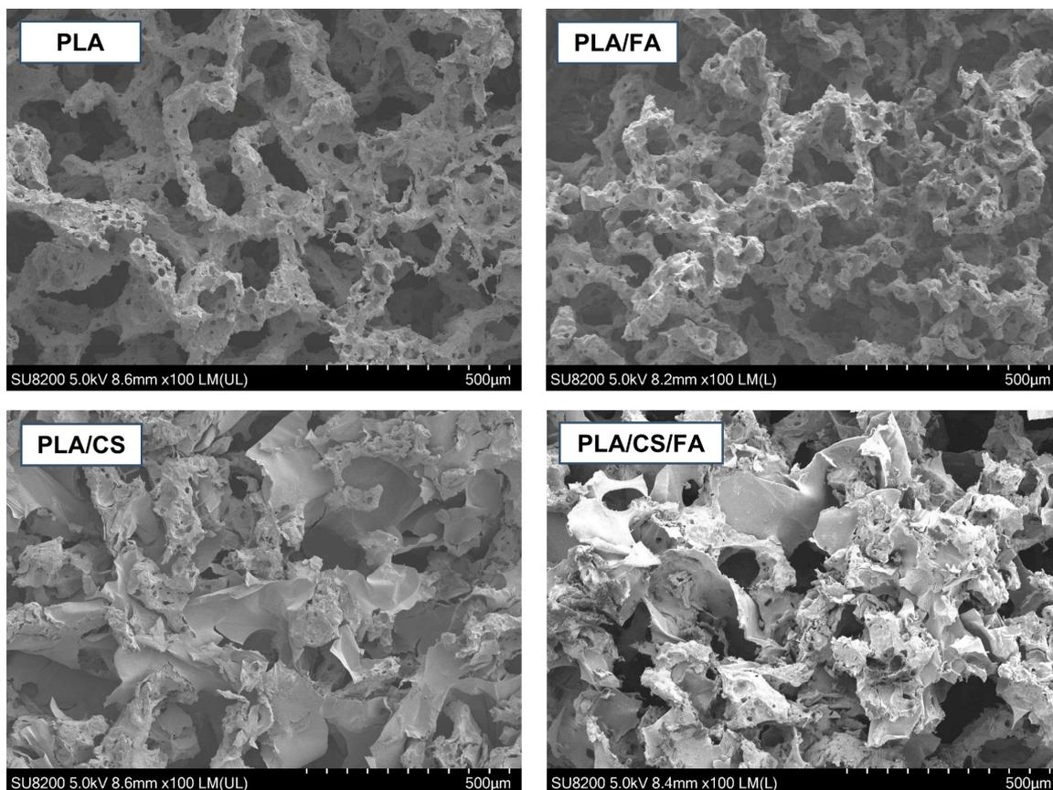
**Figure 4.** SEM images of the scaffolds cross-section.
