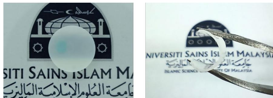
**Figure 16.** 3D-printed GPE sample.
