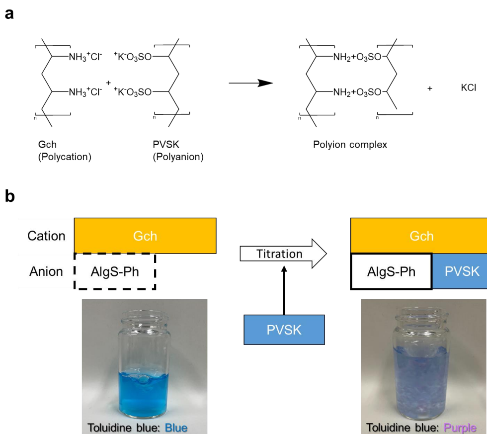
Figure S1. Colloidal titration. (a) The reaction to form polyion complex between polycation (glycol chitosan (Gch)) and polyanion (potassium polyvinyl sulfate (PVSK)). (b) schematic diagram of a titration.
