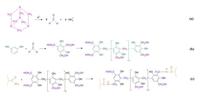
**Figure 1.** Reaction process of resorcinol /HMTA-based polymer gel. (**a**) Decomposition of HMTA into formaldehyde; (**b**) the generation of oligomers of phenolic resin; (**c**) cross-linking process between the phenolic resin and the HPAM.
