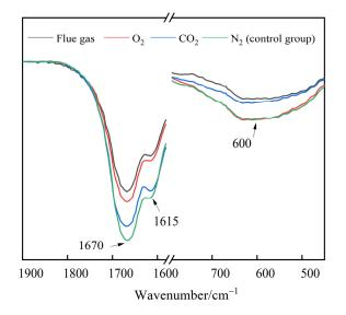
Figure 14. The FTIR spectra of polymer gel after being aged for 180 days.
