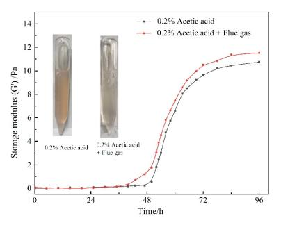
Figure 10. Gelation performance of gelant with 0.2 wt% acetic acid and flue gas.
