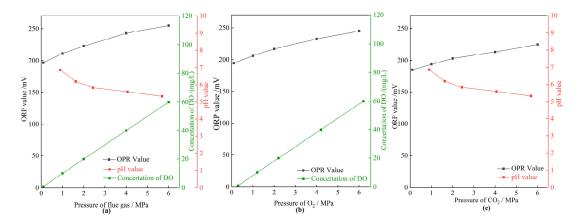
**Figure 13.** The properties of the HPAM solution in different pressures of gases. (a) The OPR value, concentration of DO, and pH value as a function of pressure of flue gas; (b) the OPR value and concentration of DO as a function of pressure of  $O_2$ ; (c) the OPR value and pH value as a function of pressure of  $CO_2$ .
