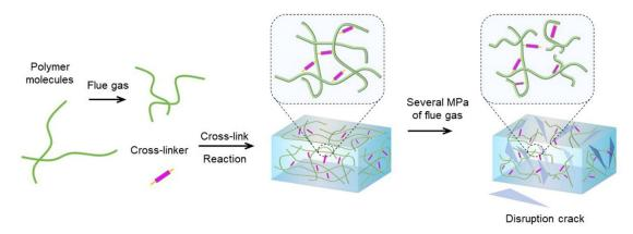
Figure 15. Schematic illustration of the generation and disruption of polymer gel in a flue gas environment.
