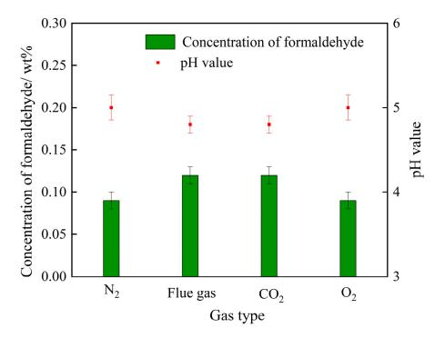
**Figure 8.** The effect of gas type on the formaldehyde concentration and the pH value of the HMTA solution.
