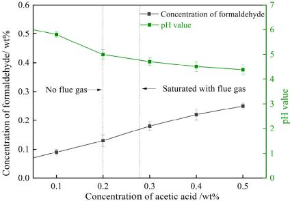
Figure 9. Effect of acetic acid on the decomposition of HMTA.
