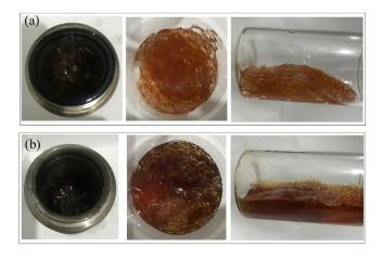
Figure 5. Gel morphology after aging for 180 days at 2 MPa. (a) Control group—N<sub>2</sub>; (b) flue gas.
