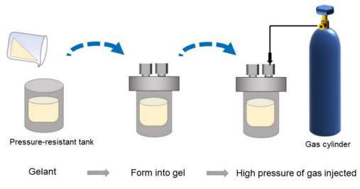
Figure 16. Experimental flow for investigating long-term stability of gels at elevated gas pressures.
