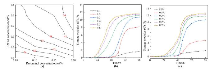
**Figure 2.** The gelation performance of resorcinol/HMTA-based polymer gel. (a) Effect of the concentrations of resorcinol and HMTA on the gelation time; (b) relationship between the storage modulus (G') of gels and the aging time as well as the mass ratio of resorcinol to HMTA; (c) effect of the concentrations of acetic acid on the gelation time.
