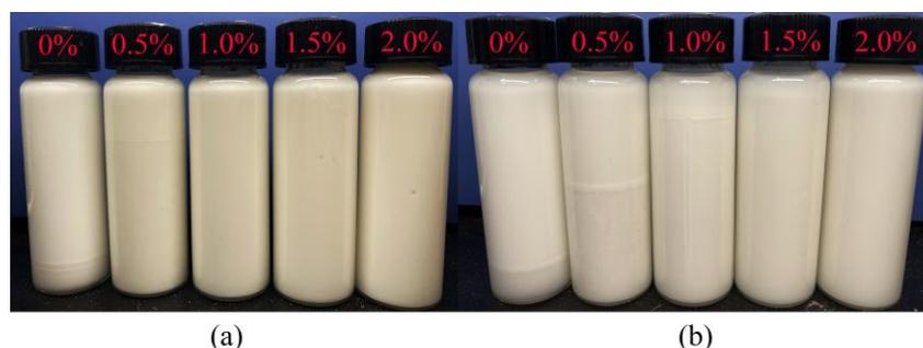
**Figure 3.** Sedimentation stability of the invert emulsions with different TQ-1 concentrations set for 1 (a) and 7 (b) days.
