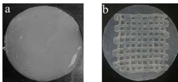
**Figure 1.** Appearance of SA/CMC-Na hydrogel membranes fabricated by our pneumatic extrusion printing system, (a) one layer as a basilar membrane and (b) three layers as a scaffold (two layers reticular scaffold and 1onelayer basilar membrane).
