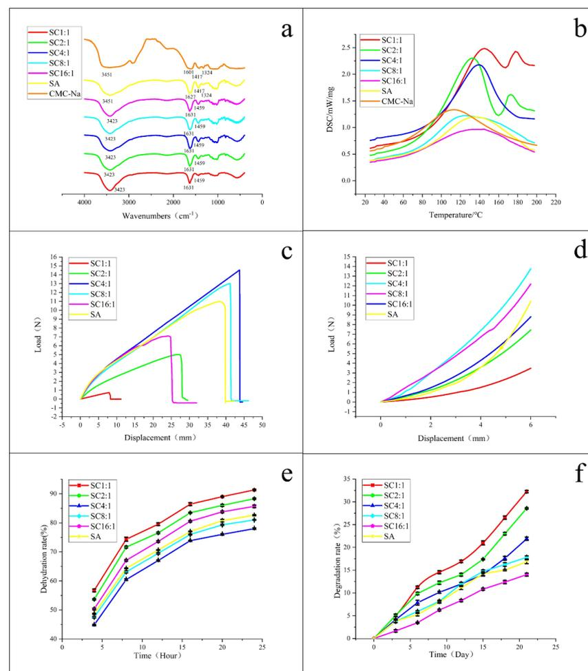
**Figure 3.** (a) FT-IR and (b) DSC curves of SC composite hydrogels; (c) tensile performance and (d) compression stress of support when compression deformation was 60% of SC composite scaffolds with different mass ratios; (e) solution viscosity test and (f) in vitro degradation rate of SC composite scaffolds with different mass ratios (each value represents the mean  $\pm$  S.D. ( $n = 3$ )).
