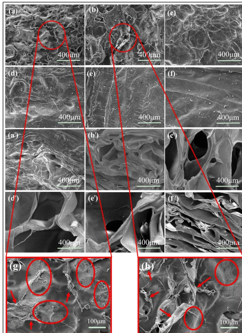
**Figure 2.** SEM images of SC composite membranes with different mass ratios at surface versions: (a) SC1:1; (b) SC2:1; (c) SC4:1; (d) SC8:1; (e) SC16:1; and (f) SA. SEM images of SC composite membranes with different mass ratios at cross-section versions: (a') SC1:1; (b') SC2:1; (c') SC4:1; (d') SC8:1; (e') SC16:1; and (f') SA. Observation surface morphology of composite scaffold with two ratios ( $\times 200$ ), (g) SC1:1, (h) SC2:1.
