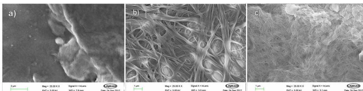
**Figure 9.** FEG-SEM images of xerogels formed by: (a) L,L,L and C8R; (b) D,D,D and C8R; (c) L,L,L + D,D,D and C8R.
