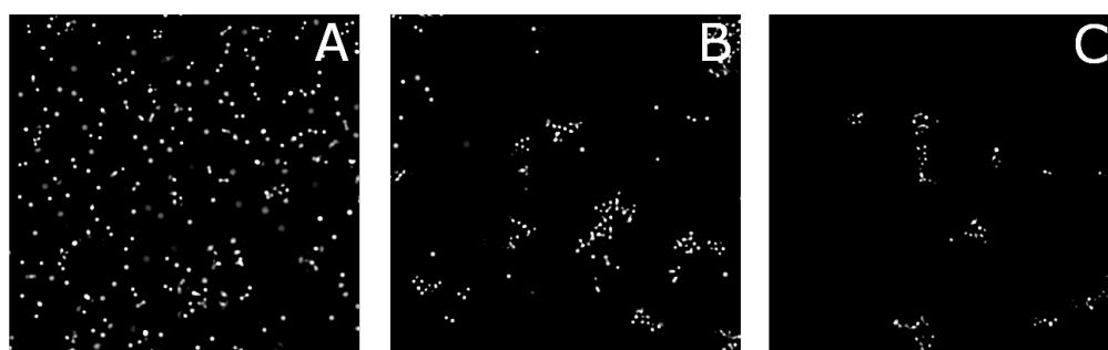
Figure 4. Optical microscopy images for different chain lengths at 32 °C in 10 mM NaCl for a grafting density of 3.0%. (A) DP = 10; (B) DP = 30; and (C) DP = 100.
