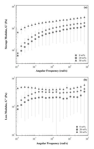
**Figure 1.** (a) Storage modulus, G' and (b) loss modulus, G" as a function of angular frequency for alginate emulsion gels prepared from emulsions with different initial silicone oil compositions.
