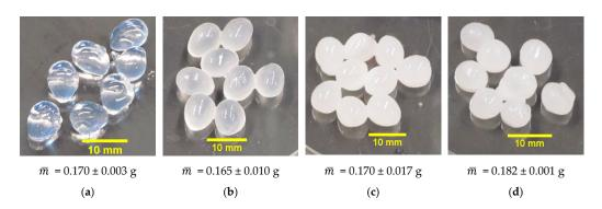
**Figure 2.** Images and the average mass per capsule,  $\overline{m}$ , of alginate capsules made from (**a**) pure alginate solution, (**b**) 20 wt% silicone oil-alginate emulsion, (**c**) 50 wt% silicone oil-alginate emulsion, and (**d**) 60 wt% silicone oil-alginate emulsion.
