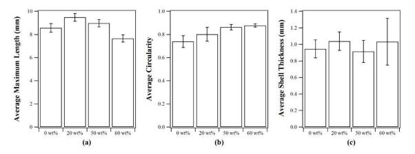
**Figure 3.** (a) Average maximum capsule length, (b) average capsule circularity, and (c) average shell thickness for capsules prepared from emulsions with different initial silicone oil compositions. Error bars represent standard deviation, n = 9.
