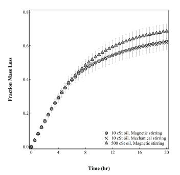
**Figure 7.** Effect of agitation method and oil viscosity on the fraction mass loss as a function of time. Error bars represent standard deviation, n = 10.
