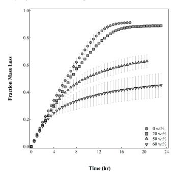
**Figure 4.** Fraction mass loss as a function of time for capsules made from emulsions with varying initial compositions of silicone oil. Error bars represent standard deviation, n = 10.
