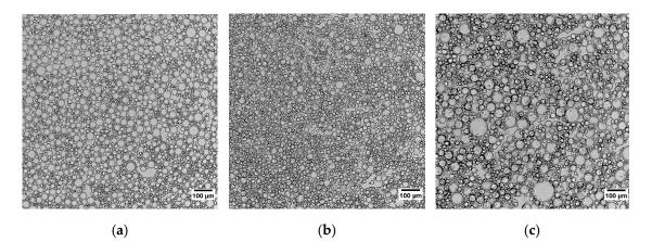
**Figure 5.** Images of silicone oil-alginate emulsions made with (**a**) 10 cSt silicone oil agitated with magnetic stirrer, (**b**) 10 cSt silicone oil agitated with mechanical stirrer, and (**c**) 500 cSt silicone oil agitated with magnetic stirrer.
