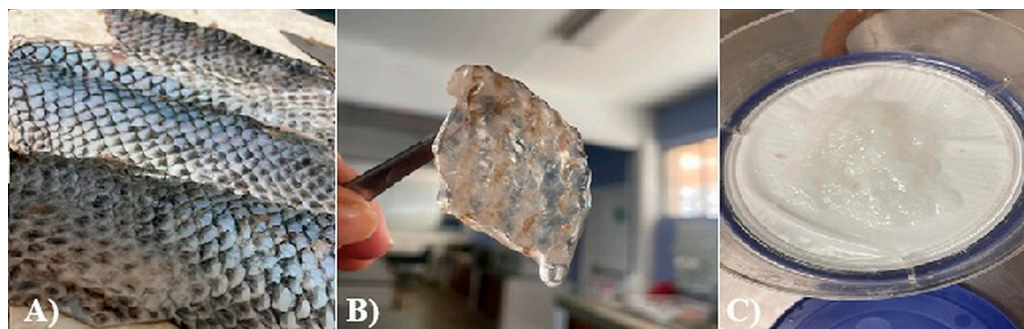
Figure 1. Collagen extraction: (A) Nile tilapia ( Oreochromis niloticus ) skin, (B) post-treatment with acetic acid, (C) marine collagen after dialysis.
