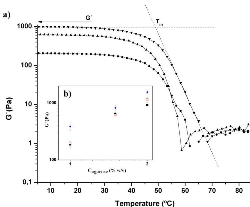
**Figure 4.** (a) Elastic modulus,  $G'$ , plotted as a function of temperature for (●) Chi/Aga-1+Fe5%, (▲) Chi/Aga-1.5+Fe5% and (▼) Chi/Aga-2+Fe5%. Dashed lines show the determination of the melting temperature,  $T_m$ , of the gel. (b) Inset image corresponds to the variation in  $G'$  as a function of agarose concentration for Chi/Aga ferrogels loaded with different concentrations of ferrofluid ((♦) 0% (w/v); (■) 2% (w/v) and (□) 5% w/v)
