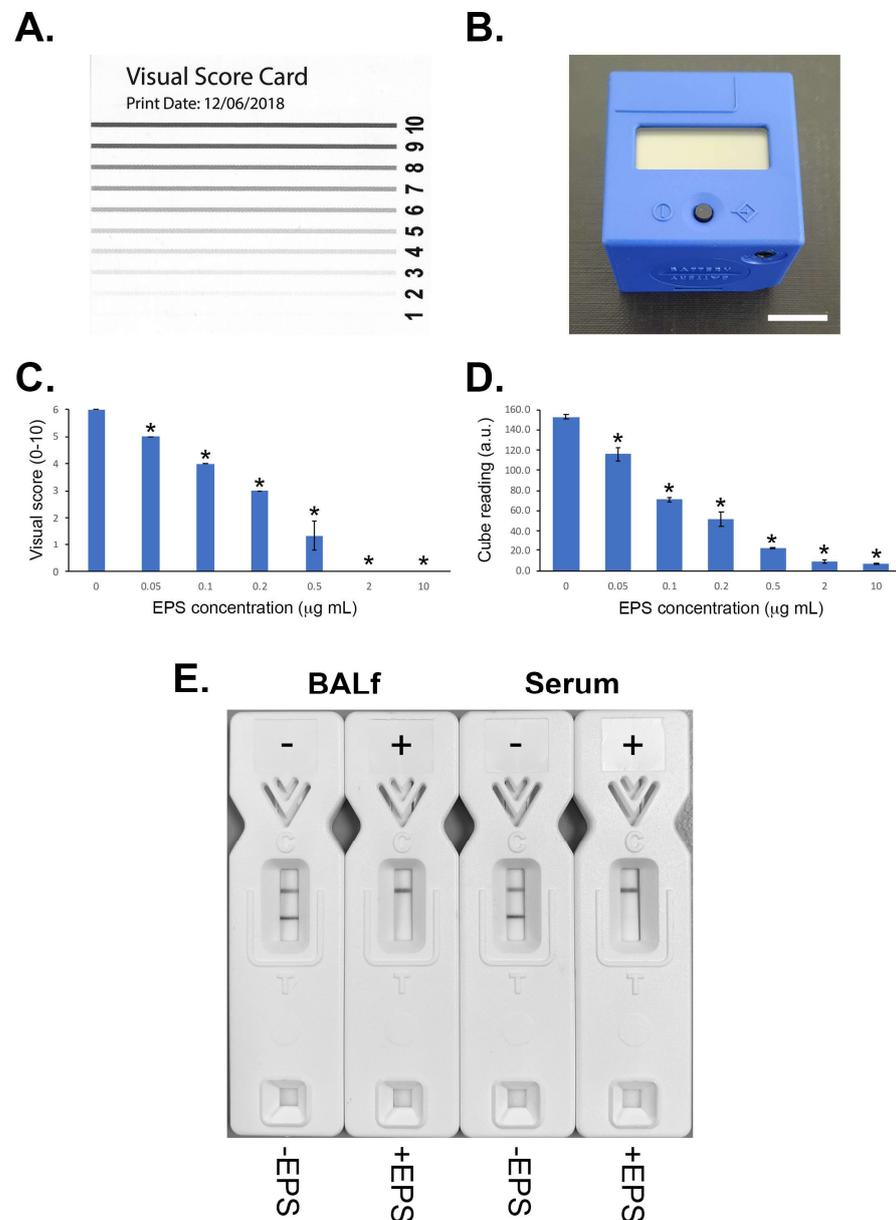
**Figure 3.** (A) Visual score card used for determinations of LFD test (T) and control (C) line intensities, recorded on a scale of 0–10. (B) Cube reader used for determination of T and C line intensities, recorded
