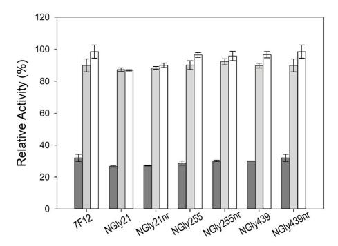
**Figure 6.** pH stability of parent laccase (7F12) and its NGly variants separated into their retained and non-retained (nr) fractions; Assay was carried out at pH 5 (dark grey bars), 7 (light grey bars) and 9 (white bars); residual activities after 24 h were measured with ABTS pH 3.
