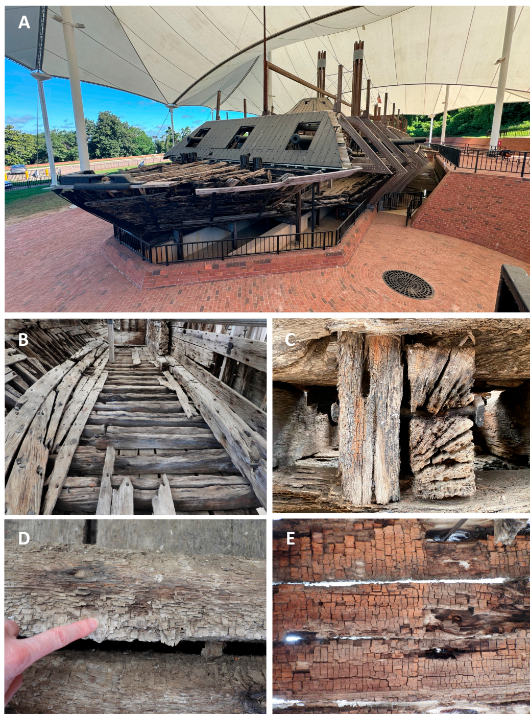
Figure 2. (A–E) The current condition of the ship and wood timbers. (A) The USS Cairo on display and under a protective canopy at the Vicksburg National Military Park in Vicksburg, Mississippi. (B,C) Ship timbers are eroded and degraded with large cracks evident. (D) White rot can be found in some woods where extensive degradation has resulted in most cells being destroyed except for the medullary ray parenchyma cells that resisted degradation. (E) Brown cubical rot typical of many brown rot fungi was found in some of the ship timbers.
