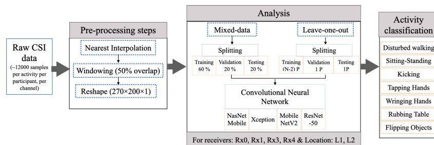
**Figure 7.** Schematic flow of agitation-based activity classification.
