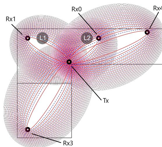
**Figure 3.** Visualization of Fresnel Zones in the experimental setup (plotting for 5.32 GHz (30th subcarrier), showing only every third zone).
