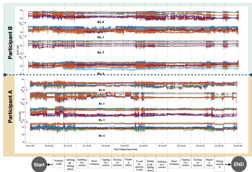
**Figure 12.** Raw CSI signal waveform from Rx0, Rx1, Rx3, Rx4. (Note that different colors correspond to different channels in the receivers).
