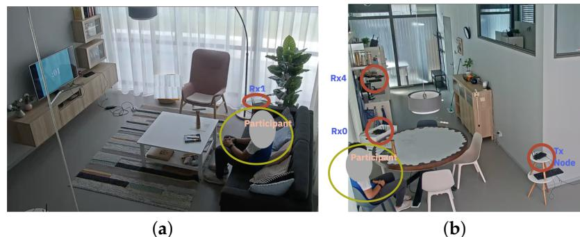
**Figure 5.** Data collection in e-health house at (a) Location 1 and (b) Location 2. The transmitter (Tx) and the receivers (Rx) placed in the living room are highlighted with red circles. Note that these images were captured from the video data obtained through cameras mounted on the ceiling of the e-health house.
