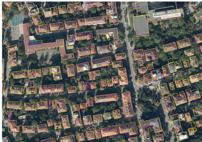
**Figure 12.** Manual adjustment of rooftop outlines in the initial approach. The yellow outlines are automatically generated, and the purple ones are manually corrected.
