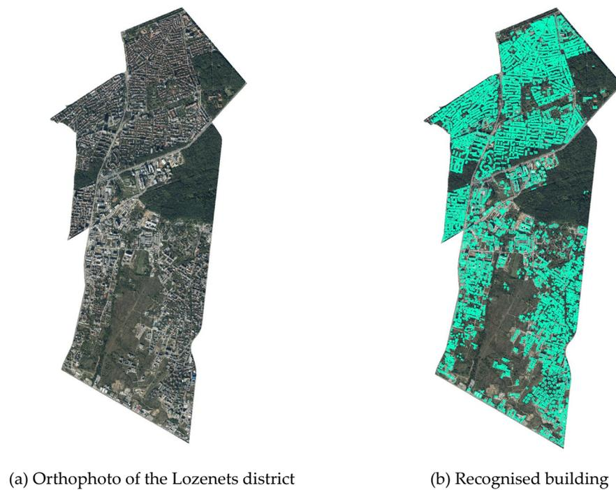
**Figure 11.** Result from the improved version, where 3834 objects are recognized as buildings. (a) Orthophoto of the Lozenets district; (b) Distribution of the recognized building by Mapflow.
