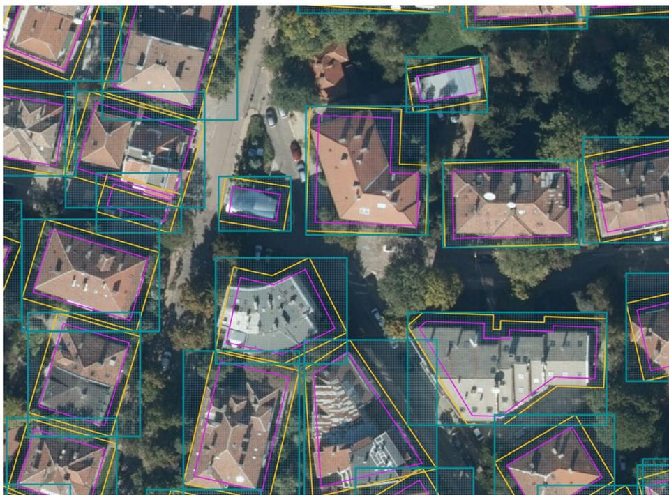
**Figure 15.** Bounding boxes (green), generated according to the buffer outlines (orange).
