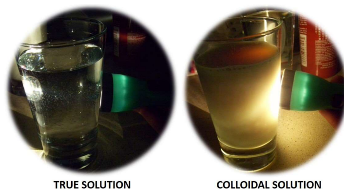
Figure 2. The Tyndall effect [9]. When light is shined through a true solution, the light passes cleanly through the solution, however, when the light is passed through a colloidal solution, the substance in the dispersed phases scatters the light in all directions, making it readily seen.
