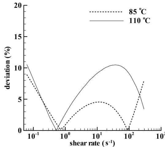
**Figure 4.** The deviations between the  $N_1$  calculations with the power law strain model and those with the linear strain model for two kinds of corn starch dispersions. One is heated to 85 °C in the Rotavapor, and the other is in cans at a retort temperature of 110 °C.
