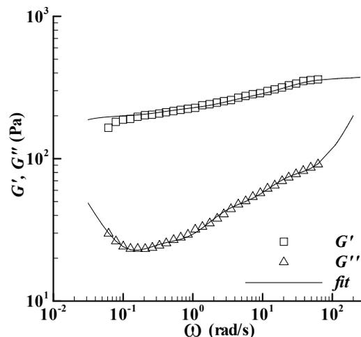
**Figure 1.** The linear viscoelastic property of the cross-linked waxy corn starch dispersion at 20 °C, which is mixed with 300 g/kg sucrose and heated to 85 °C in the Rotavapor. The symbols are the experiments in Figure 7a of Acquarone and Rao [18], and the lines are the fits here.
