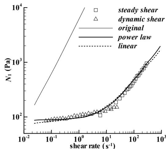
**Figure 3.** First normal stress difference of the cross-linked waxy corn starch dispersion at 20 °C, which is mixed with 300 g/kg sucrose and heated to 85 °C in the Rotavapor. Symbols are the ex-
