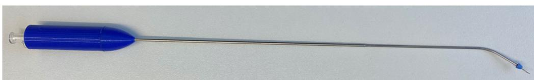
**Figure 1.** Injection instrument with the retractable cannula being pushed forward.
