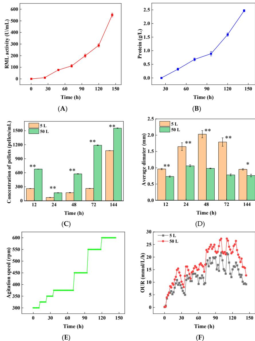
**Figure 6.** The RML activity (A), protein concentration (B), pellet concentration (C), pellet diameter (D), agitation strategy (E), and OUR (F) in 50 L bioreactor. \* indicates  $0.01 < p < 0.05$ , \*\* indicates  $p < 0.01$ . Data expressed as the mean  $\pm$  standard deviation ( $n = 3$  per group, per time point).
