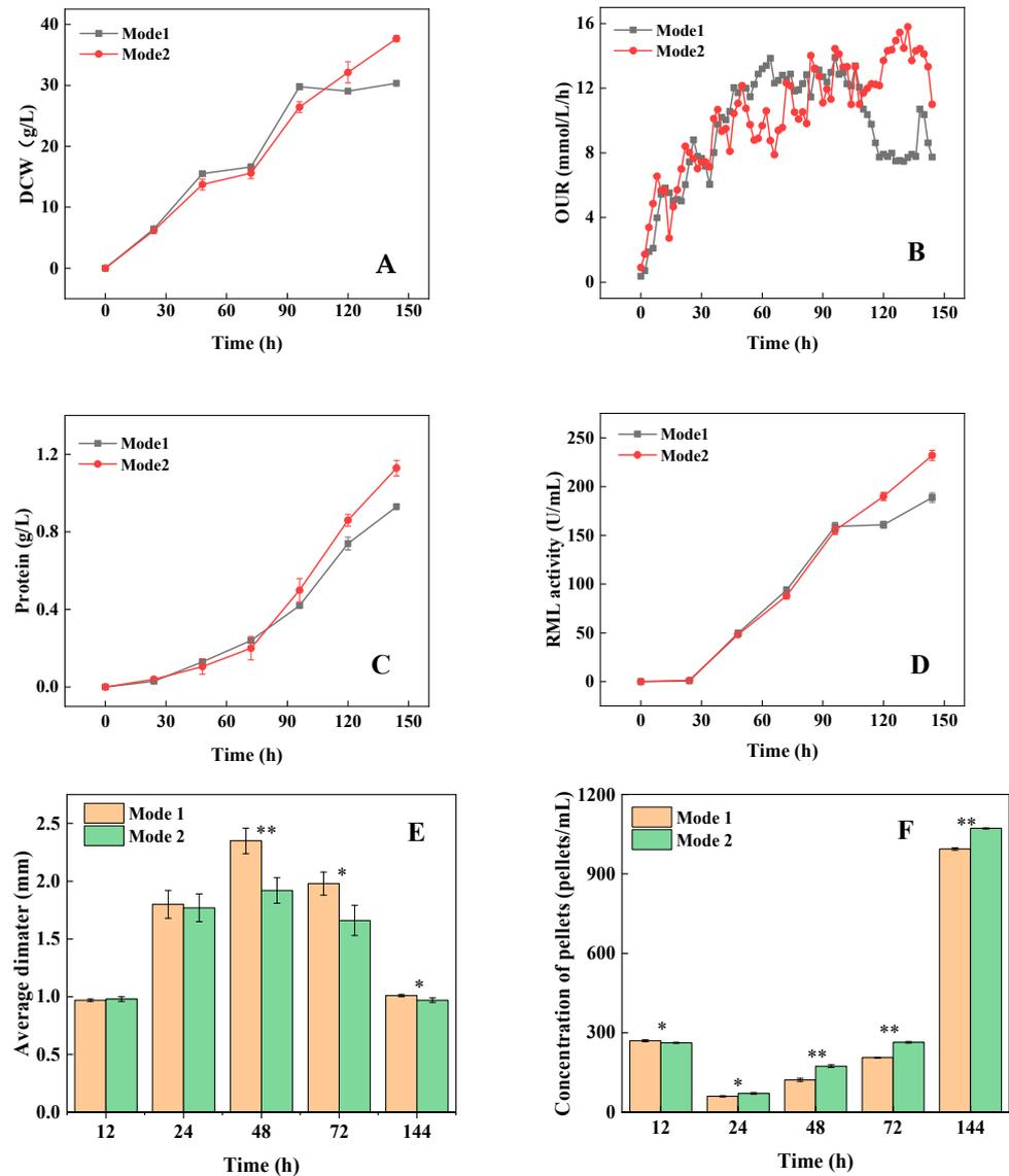
**Figure 4.** Comparison of DCW (A), OUR (B), protein (C), RML activity (D), average pellet diameter (E), and pellet concentration (F) with different agitation strategies. \* indicates  $0.01 < p < 0.05$ , \*\* indicates  $p < 0.01$ . Data expressed as the mean  $\pm$  standard deviation ( $n = 3$  per group, per time point).
