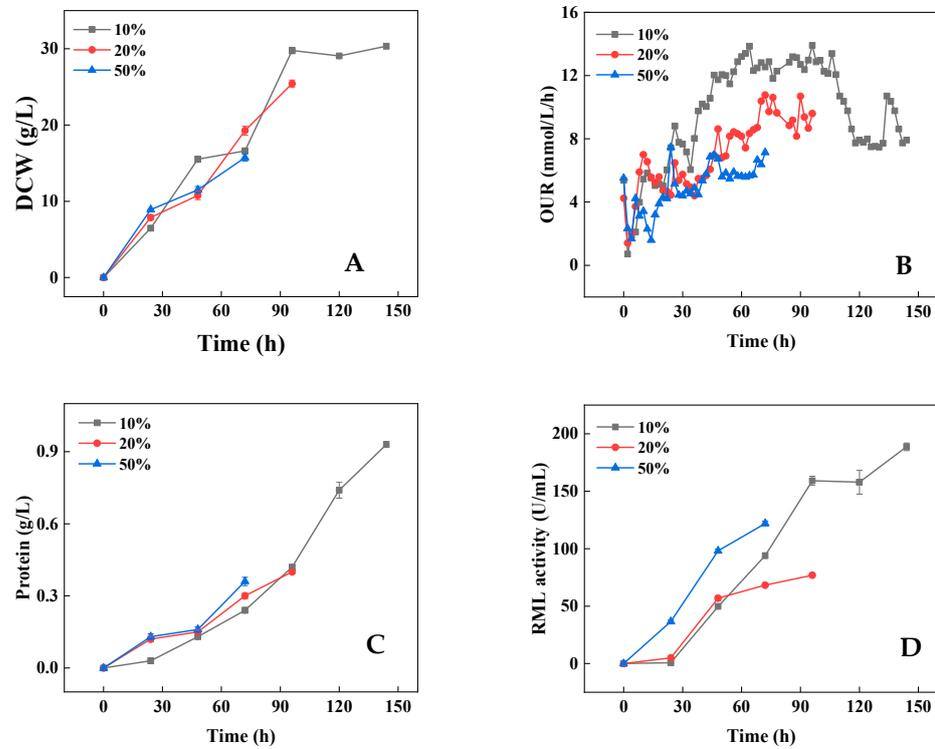
**Figure 3.** Cell growth (A), OUR (B), protein synthesis (C), and RML production (D) under different initial nitrogen source conditions. Data expressed as the mean  $\pm$  standard deviation ( $n = 3$  per group, per time point).
