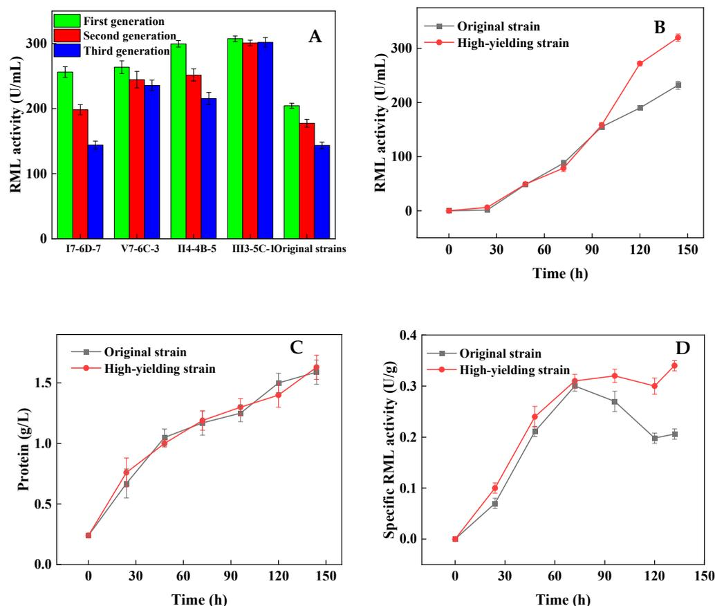
**Figure 5.** Comparison of the RML activity by different strains (A) in shake flasks, and the comparison of RML activity (B), protein concentration (C), and specific RML activity (D) between the high-yield strain and original strain in 5 L bioreactor. Data expressed as the mean ± standard deviation (n = 3 per group, per time point).
