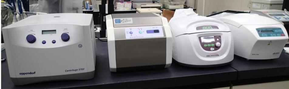
**Figure 2.** Major centrifuges used for PRF preparation. From left to right: Eppendorf #5702 (for BIO-PRF), Medifuge (for CGF), Duo Quattro (for A-PRF), and Hettich EBA200 (original model of Intra-Spin) (for L-PRF).
