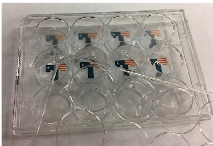
**Figure 1.** Physical appearance of the four polyurethane (PU) films: From left to right in the top wells, 200ET, 100ES, 60ES, and 60ET. The second row of four wells contains no PU films for comparison of the transparency of the PU films.
