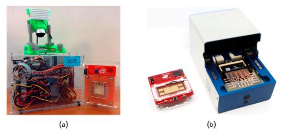
**Figure 14.** Direct comparison in size between (**a**) DropBot version 1 and OpenDrop version 1, and (**b**) OpenDrop version 3 and DigiBio instrument. The Dropbot photo is from R. Fobel and used with permission.
