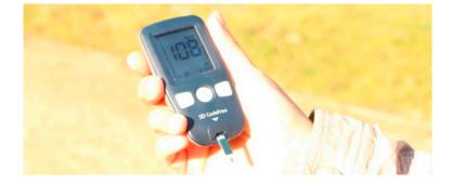
**Figure 4.** A glucose meter is a commercial instrument that uses capillary microfluidics to measure glucose levels in blood droplets. It is operated from a battery and can be used in mobile scenarios.
