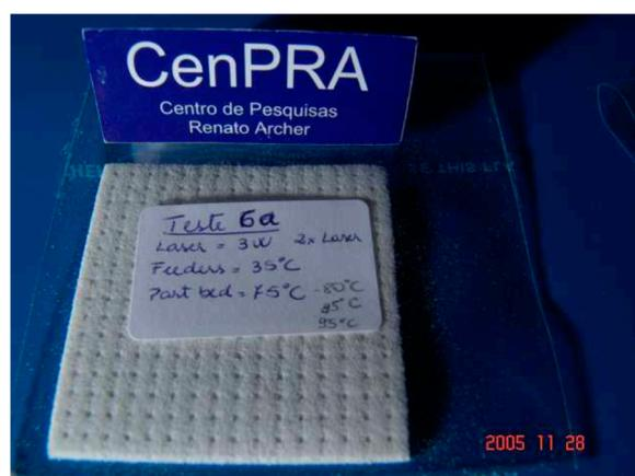
**Figure 6.** Sintered PHB using SLS containing pores of 1 mm in diameter [66].
