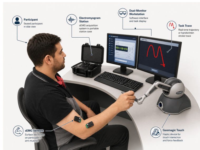
Figure 3. Representative experimental configuration. The participant manipulated the Geomagic Touch stylus while viewing the target trace on a dual-monitor workstation. Wireless sEMG sensors recorded upper-limb activity.
