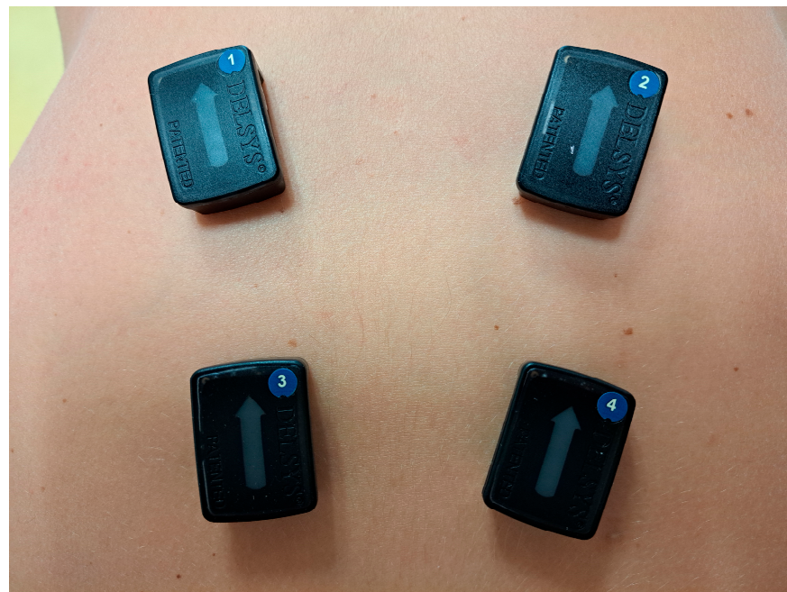
Figure 3. Example of multi-channel EMG (polyEMG) electrode placement on the lower back. Illustrative placement of four bipolar electrode pairs along the lumbar region to capture spatial differences in activation across segments. Multi-channel EMG can be synchronized with kinematic sensing (e.g., IMU) to relate muscle activation strategies to movement execution during functional tasks and rehabilitation. In our feasibility experiments, EMG was acquired using commercially available wireless systems (Shimmer and Delsys); the focus was on long-duration recording and the acquisition/analysis pipeline to assess signal quality and practical feasibility over extended monitoring, rather than on developing new hardware.
