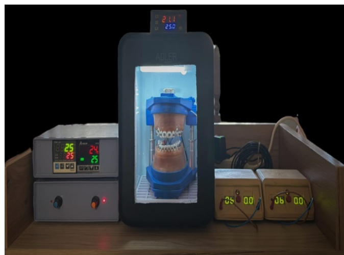
Figure 1. Scientific orthodontic simulator with temperature control and thermo controlled chamber.
