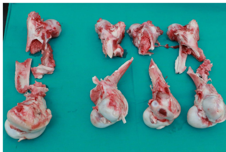
Figure 9. Photos of FEMUR bone after impact test, velocity of 10 m/s.
