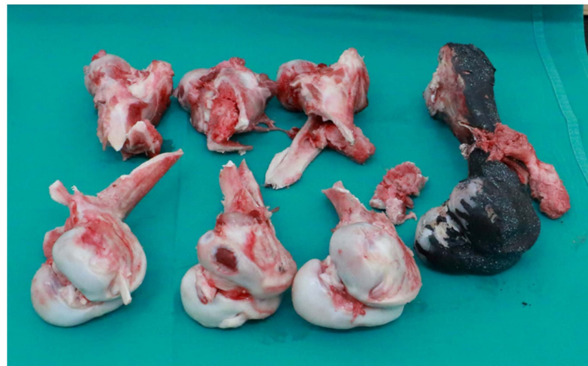
Figure 6. Photos of FEMUR bone after impact test, velocity = 5.15 m/s.
