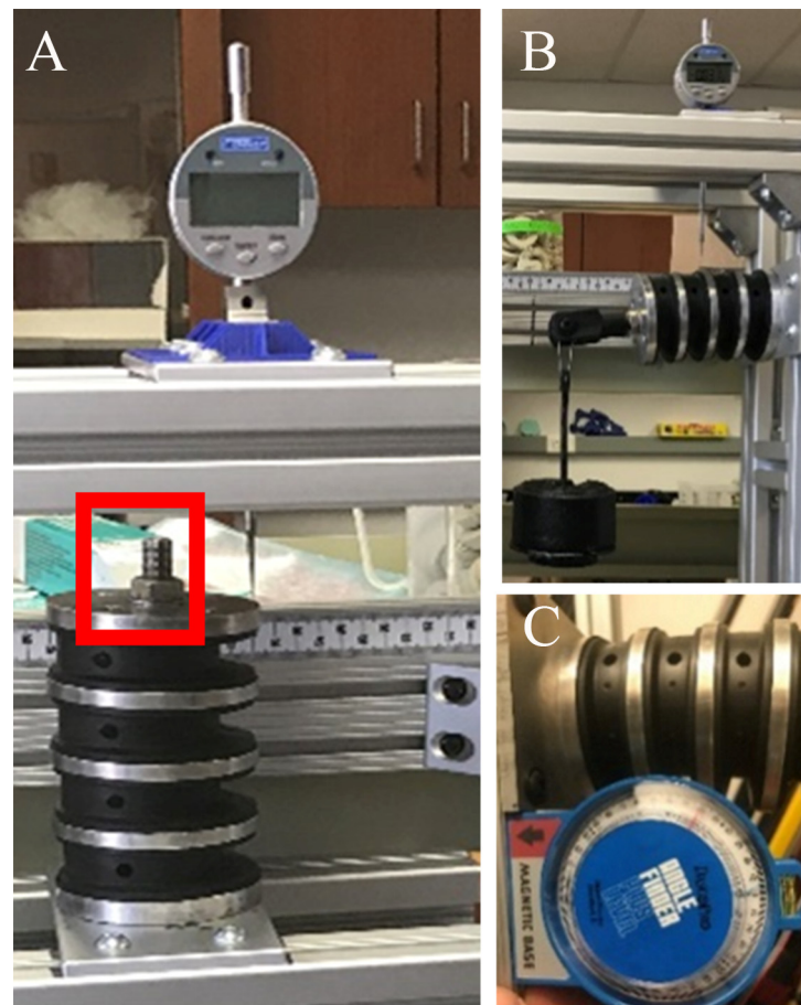
Figure 3. Hybrid III neck calibration. (A) Dial indicator being used to measure Hybrid III neck compression. (B) weights being mounted on the Hybrid III neck to measure stiffness. (C) Hybrid III neck deformation is being measured using a protractor.
