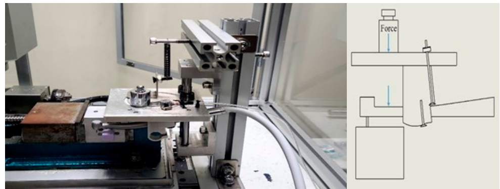
Figure 10. Picture of the DATH, glass porcelain block (purple color), attached accelerometer, and applied 100 g force, as illustrated on the right.
