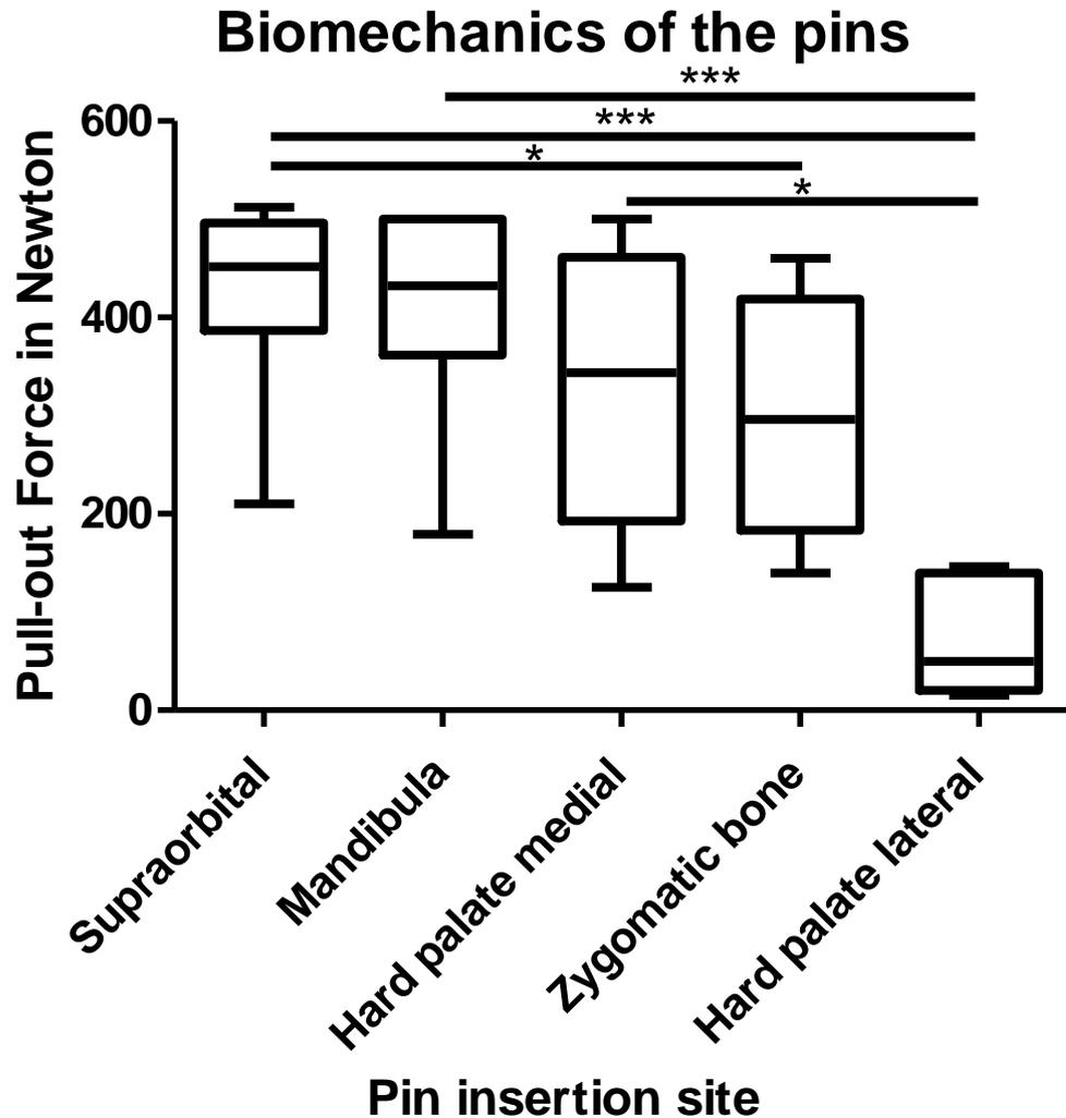
**Figure 3.** Evaluation of the pull-out forces of the EFF pins using an ANOVA analysis with Kruskal–Wallis and Dunn’s multiple comparison tests. Significance level: (\*\*\*)  $p < 0.001$ , (\*)  $p < 0.05$ . All other pull-out forces were not significantly different.
