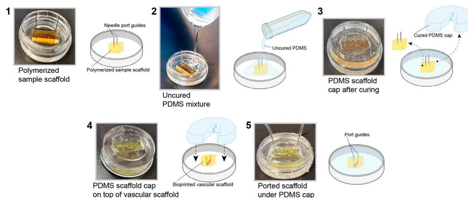
**Figure 2.** Fabrication of a PDMS cap to perfuse the 3D bioprinted scaffold. A PDMS cap was fabricated using the soft lithography technique. The completed polymerized PDMS cap was applied to the top of the scaffold to support placement of the needles for perfusion.
