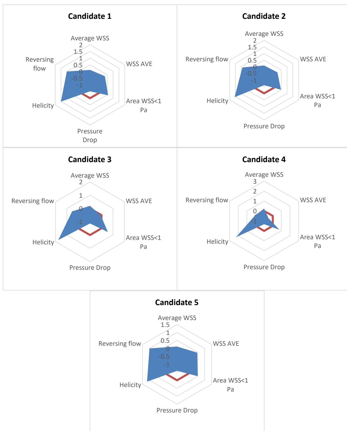
Figure 2. Comparison of the different candidates' performances compared with the reference case with no ridge (red line): positive values denote improved performance compared with the reference solution. Please refer to Table 4 for the scale/numbers shown in each figure.
