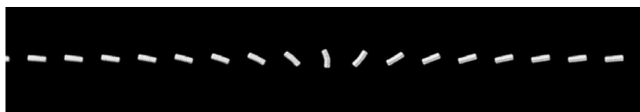
Figure 11. Microrods of 400 \mu\text{m} length rotating along the needle (needle size 0.8 mm, flow rate: 100 \mu\text{L}/\text{min} ).
