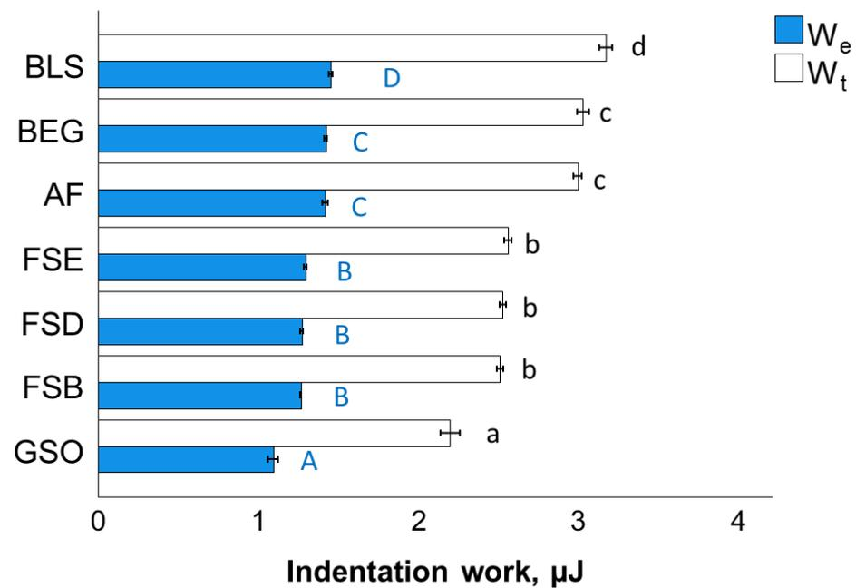
**Figure 9.** Elastic ( $W_e$ ) and total indentation work ( $W_t$ ) as a function of RBC and aging conditions (mean values with 95% confidence interval; capital and small letters indicate statistically homogeneous subgroups; Tukey’s HSD test,  $\alpha = 0.05$ ). Material abbreviation: AF = Admira Fusion; BEG = Brilliant EverGlow; BLS = Beautifil II LS; FSB = Filtek Supreme XTE Body; FSD = Filtek Supreme XTE Dentin; FSE = Filtek Supreme XTE Enamel; GSO = Grandio SO.
