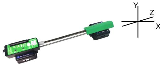
Figure 8. IMU system and goniometer.
