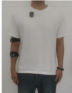
**Figure 10.** Wearing position of the IMU system.
