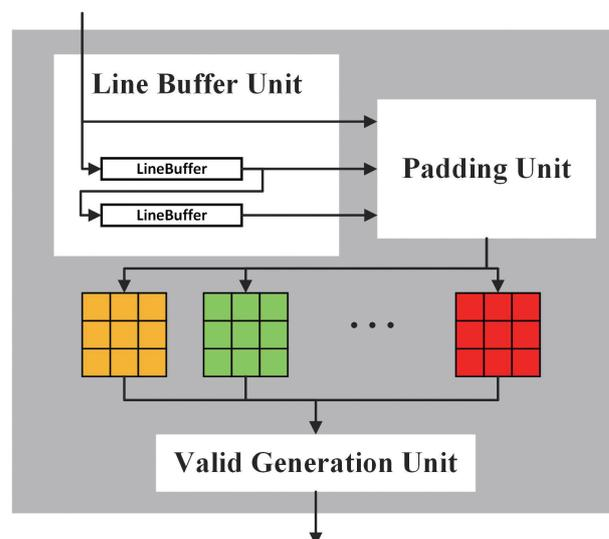
Figure 6. DWC Accelerator architecture.
