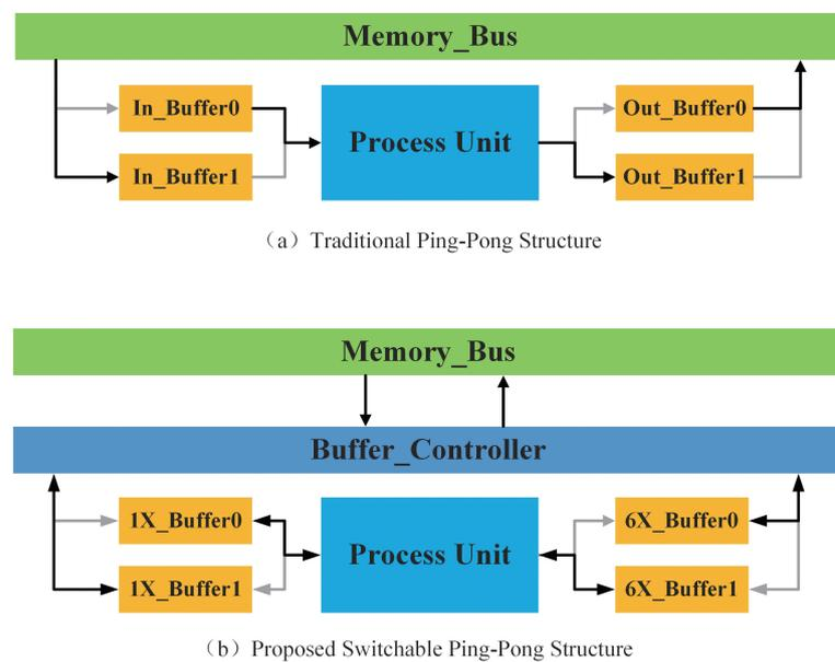
**Figure 8.** On-chip memory architecture.
