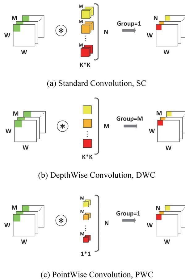
**Figure 1.** Standard convolution and depth separable convolution.
