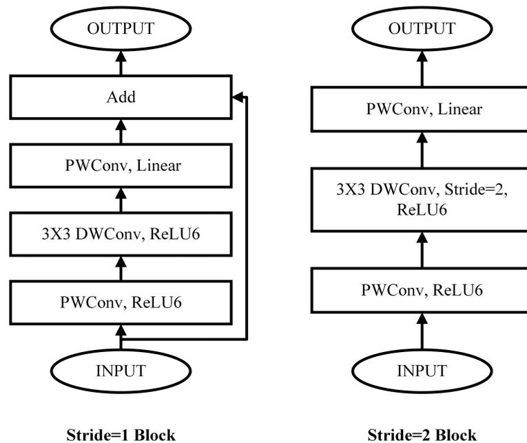
Figure 3. MobileNetV2 basic block.
