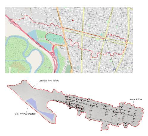
**Figure 10.** Case 3: Map of the considered area with the domain limitation (**upper**) and position of the 147 surface-sewer links (**lower**). Surface boundary conditions and sewer inflow is also depicted.
