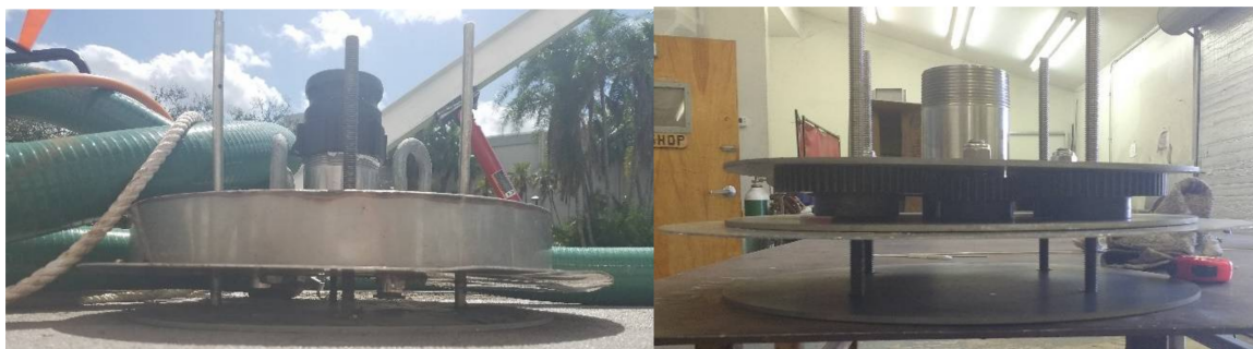
Figure 2. Variable area suction head (with and without gearbox cover, shown left to right).
