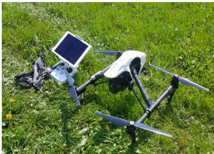
Figure 2. UAV platform DJI Inspire 1 Pro, used for monitoring campaigns. Photo by J. Langhammer.
