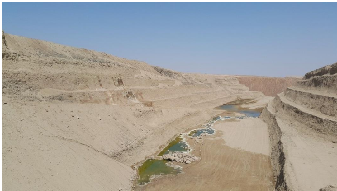
Figure 5. Seepage outlet at Langerheinrich Uranium Mine.
