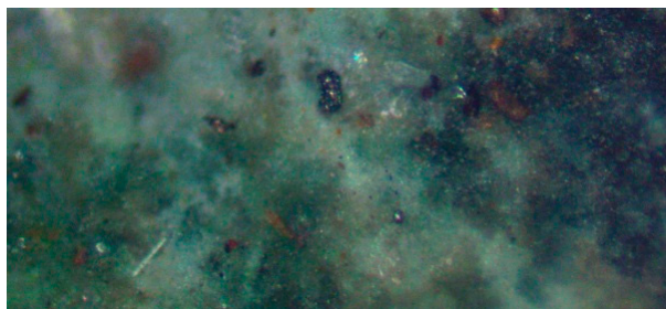
Figure 3. ST Trial Pellet (ST1b [16]) Following Desalination: Reflected Light; Halite infilling porosity on polished cut surface. Field of view = 0.49 mm; ZVI:water ratio = 23.10 g/L; Feed water salinity = 8.21 g/L; Product water salinity after 230 days = 1.99 g/L. NaCl removed = 6.22 g/L (0.27 g/g ZVI). Feed water pH = 6.25; Product water pH = 8.15.
