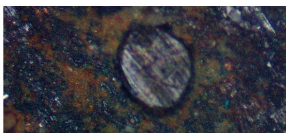
Figure 4. ST Trial Pellet (ST1c [16]) Following Desalination: Reflected Light; Halite infilling circular pore on polished cut surface. The halite infilling the circular carrier pore shows a characteristic “kristallbrocken” texture [49] indicating that the pore was infilled by crystal masses growing out from the pore boundaries. The bulk of the matrix in the photomicrograph is constructed from goethite [41–48]. All the pores are infilled with halite. The blue lath shaped crystals are atacamite. Field of view = 0.52 mm; ZVI:water ratio = 25.34 g/L; Feed water salinity = 8.19 g/L; Product water salinity after 230 days = 2.28 g/L. NaCl removed = 5.91 g/L (0.23 g/g ZVI). Feed water pH = 6.21; Product water pH = 8.54.
