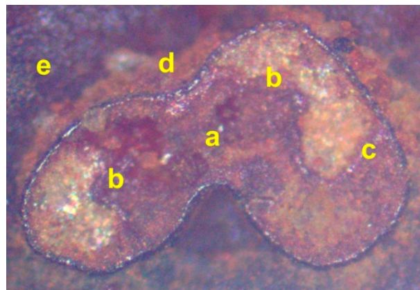
Figure 14. Trial ST1e [16] ZVI desalination pellet following desalination. (a) = authigenic oolitic goethite nodule; (b,c) = adsorbed oolitic goethite nodules containing authigenic cuboid Fe 0 crystallites (1 to 5 microns in diameter) crystallizing within the goethite. The Fe 0 crystallites vary in color from white to blue to yellow to pink (depending on orientation), are cuboid, isotropic, and have a reflectance of about 60%. Sub-nodule (c) includes a rim of (FeO (wustite) with exsolved Fe 0 crystals) separating it from the main goethite (FeO(OH)) mass of the nodule; (d) = iron rich boundary of the nodule (FeO (wustite) with exsolved Fe 0 crystals) and the associated active outer growth fringe (light brown) of the oolitic nodule. (e) = goethite matrix (dark). Reflected light. Field of view = 0.173 mm; ZVI:water ratio = 21.72 g/L; Feed water salinity = 8.22 g/L; Product water salinity after 230 days = 2.24 g/L. NaCl removed = 5.98 g/L (0.28 g/g ZVI). Feed water pH = 6.24; Product water pH = 8.42.
