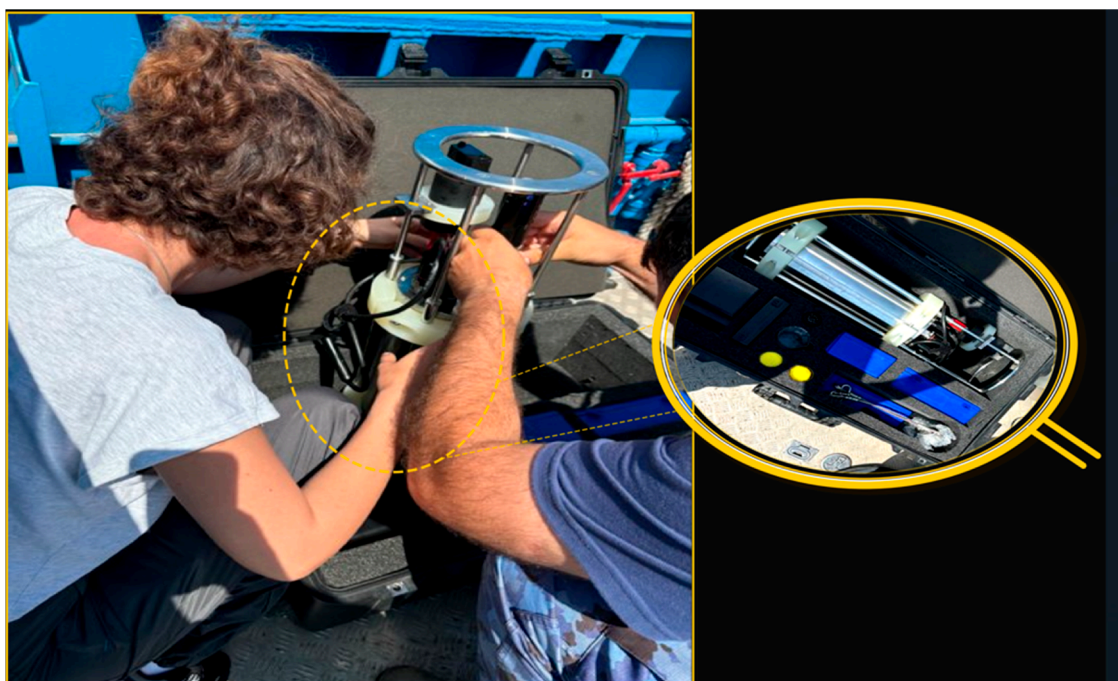
Figure 2. Midas CTD+ instrument.
