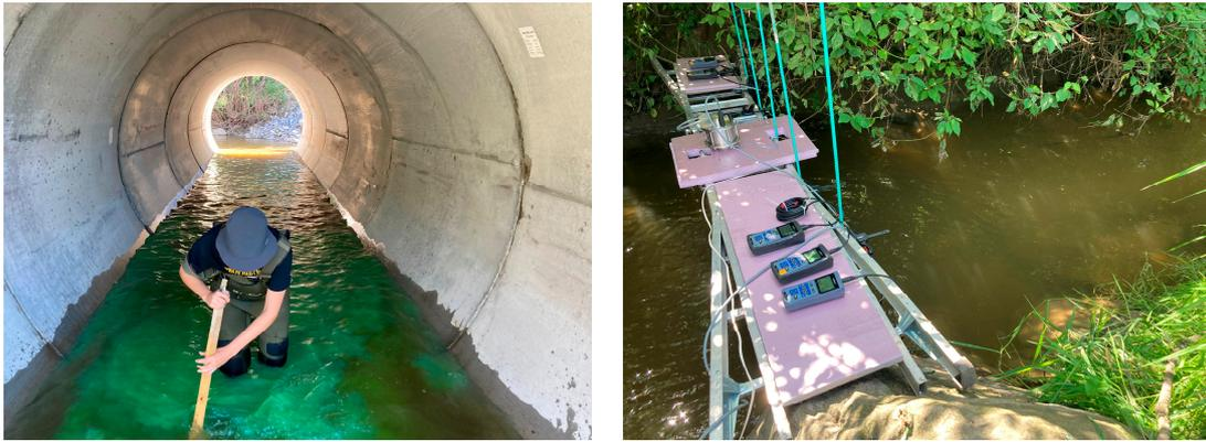
**Figure 2.** (On the left): picture of the stream at the injection site (under a small culvert). We ensured tracer homogeneity by manually fanning the water under the culvert. (On the right): picture of the restitution site with the equipment used to monitor solute concentration.
