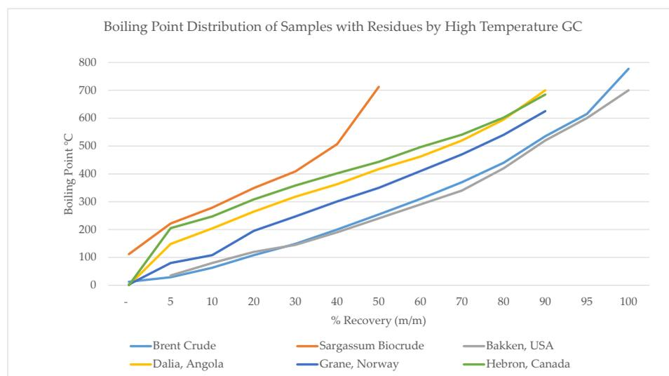
**Figure 2.** Boiling point distribution (ASTM D7169) of HTL oil from Mexican *Sargassum* seaweed compared to other common petroleum fractions.
