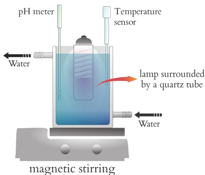
**Figure 3.** Photochemical reactor bench illustration.
