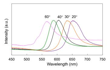
Figure 4. Angle dependance of PBG for silica opal (opal-295).
