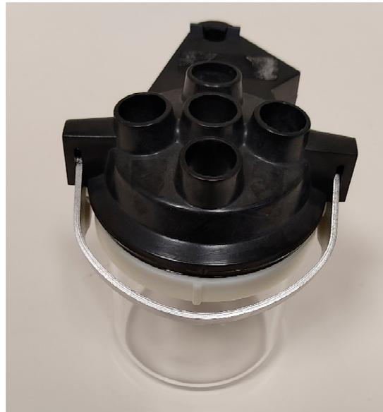
**Figure A1.** A sealed beaker with inlet holes for electrodes and for the acid titration tubing.
